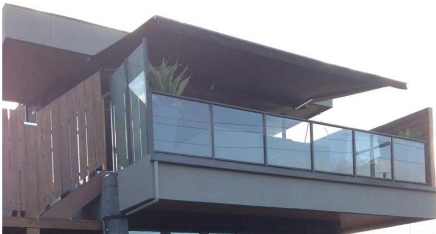
The good thing about this system and the other new systems we've just released is that they're all rated up to a 50km/h wind rating and this particular awning we can make up to 14 metres wide with a 3.6 metre extension, now, that is absolutely huge. We can also adjust the angle or the pitch that the folding arm comes in and comes out. This particular system here can go from 5 degrees down to 85 degrees, giving you all the options that you need.
